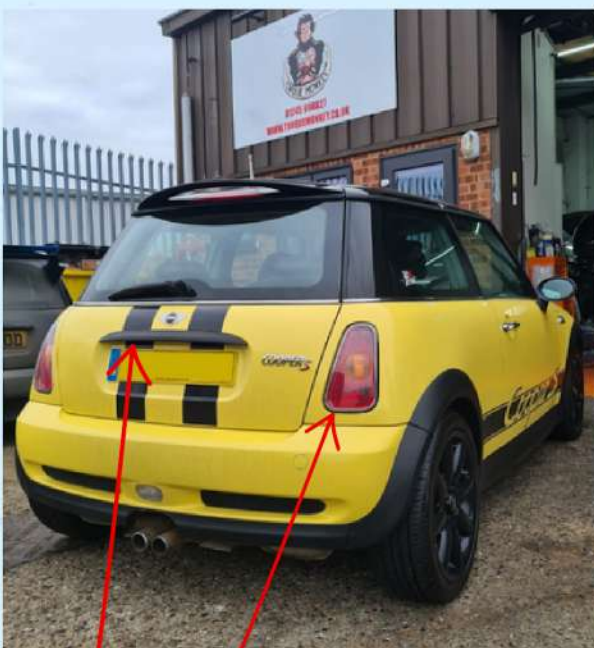
Areas for common rust on car exterior
